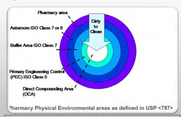
A decreasing pressure gradient continuously moves the air from the buffer-room toward the ante-room and then toward the line of demarcation, the gowning area and exit door.
